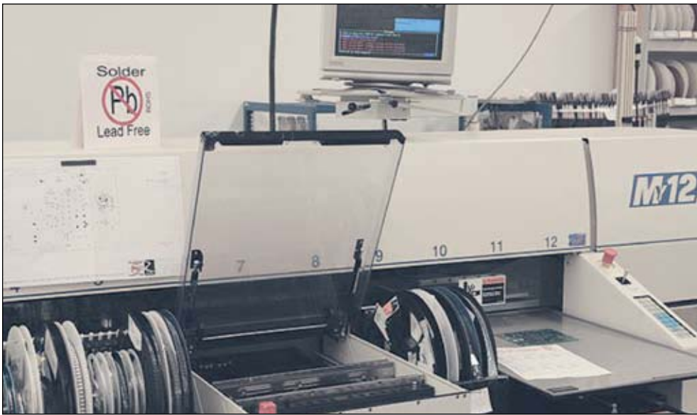
Dual-use SMT line set up to build lead free assemblies.
