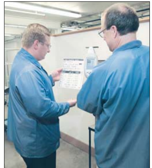
(From left) Keith Crane and Scott Wilson evaluate components' RoHS compliance using a Niton XRF analyzer.
